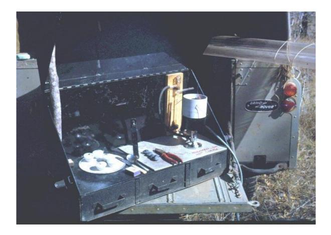
Field Coal Swell Testing Kit - circ 1960
